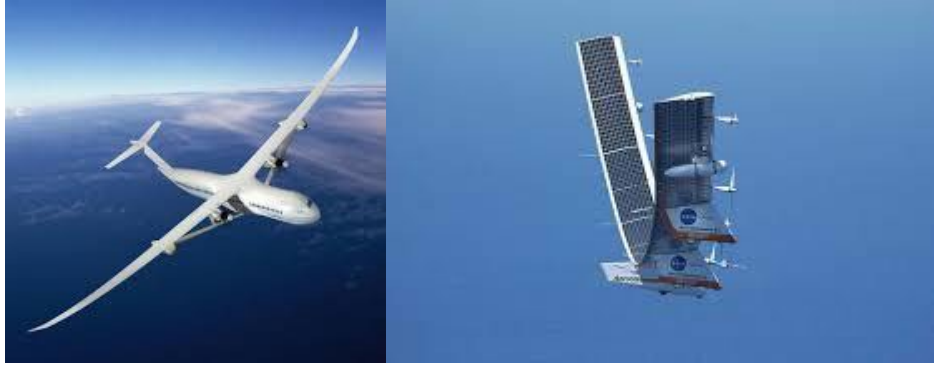
Figure 1 - High-aspect-ratio wing designs: Boeing SUGAR volt concept plane (Left), NASA Helios (right)
